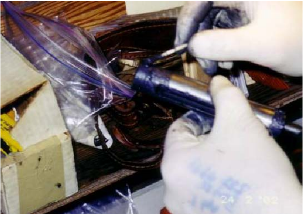
Beeman moly grease being applied to the piston seal sides. Note the moly grease already applied to the rear skirt of the piston. Surgical gloves keep the hands clean and help protect against minor cuts.
