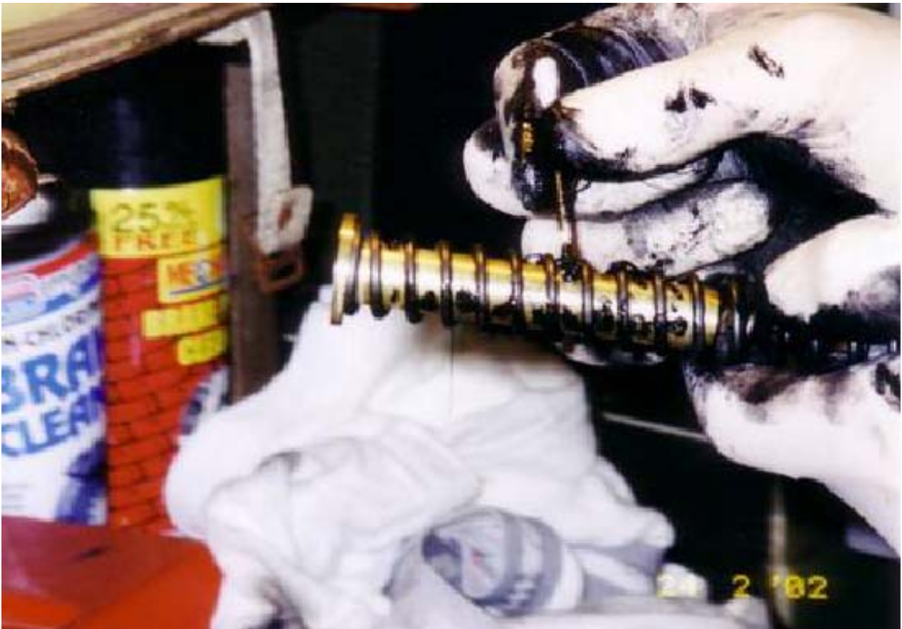
Maccari velocity tar being applied to the mainspring and rear guide of a Maccari tune kit for a HW55.
