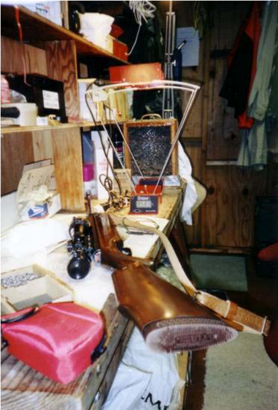
A chronograph is a valuable tool to check the health of your air rifle. Here Robert checks the velocity of his FWB124d.
