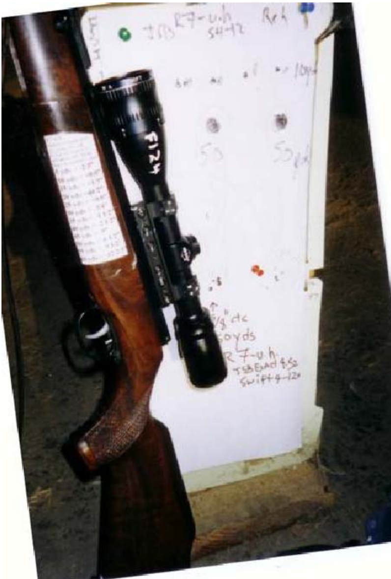
Robert's Beeman R7. Note the pistol grip checkering, but no forearm checkering. The pistol grip should always be checkered or at least stippled on a hunting air rifle for a secure grip. No need for forearm checkering when the Artillery Hold is used.
