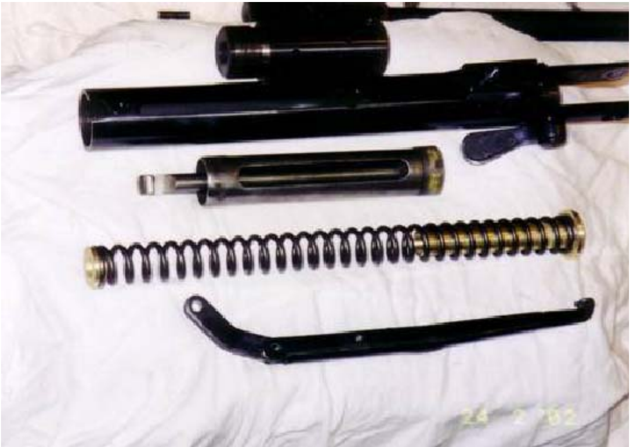
A Weihrach HW55 disassembled and undergoing installation of a Maccari mainspring & guid set.
