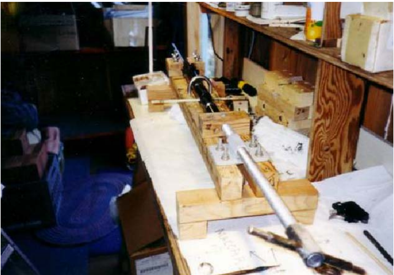
Robert's Randy Gunn model spring compressor. Built from plans available at Randy's web site, it's affordable and a valuable tool for experienced "do it yourself" springer owners.
