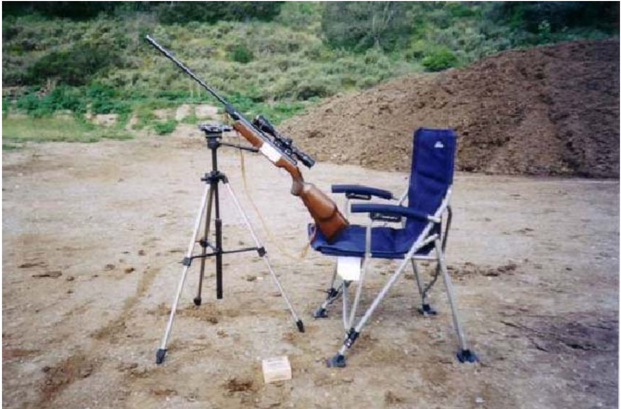
Tom Jue and I use this set up for our target shooting/trajectory plotting: folding camp chair and camera stand with heavy plexiglass 4"x5" plate on top to rest the hand on. Black tape holds the pad on top the plexiglass. Light and mobile setup.
